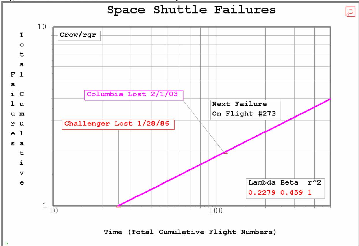
Figure 3 forecasts the next shuttle failure at flight number 273 based on the extrapolated trend line where the line crosses failure #3. Figure 3's line slope shows beta = 0.459 which tells of
