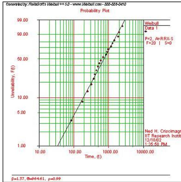
Figure C-5. Graph of Weibull plot from Weibull++<sup>TM</sup> for data analysis example.
