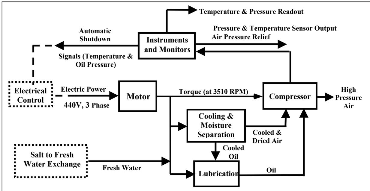
Figure 4-1. Example of a functional block diagram.
