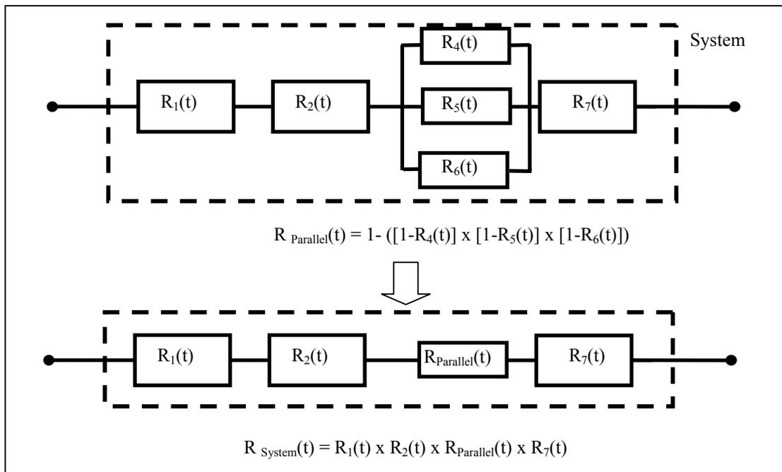
Figure 3-7. Calculating the reliability of a combined configuration.
