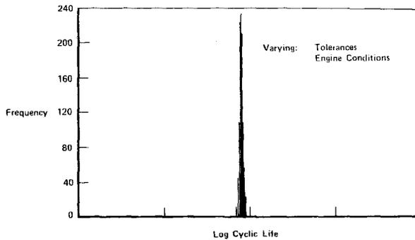
Fig. 10 1st Turbine Disk Life Distribution Holding Material Properties at Mean.
