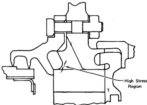
Fig. 6 The LCF Limiting Location Occurs in Cooling Passage Through Disk Rim.
