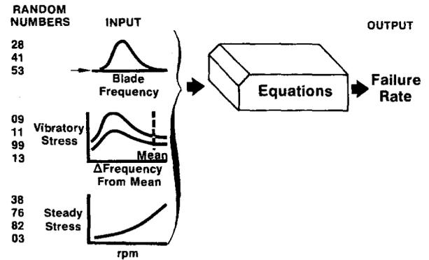
Fig. 11 Monte Carlo Simulation of 2nd Turbine Blade Failure.
