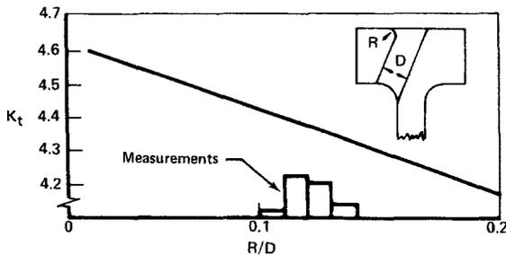
Fig. 7 Effect of Dimensional Control on Hole on the Stress Concentration Factor ( $K_t$ ).
