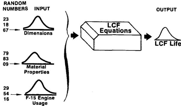
Fig. 5 Monte Carlo Simulation of First Turbine Disk.
