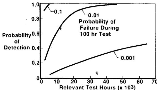
Fig. 1 Failure Mode Detection.
