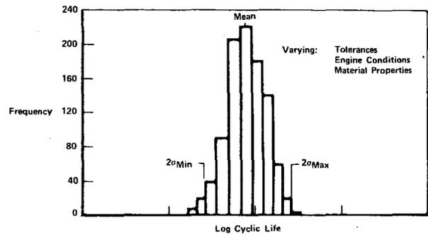
Fig. 9 1st Turbine Disk Cyclic Life Distribution of 1000 Engines.
